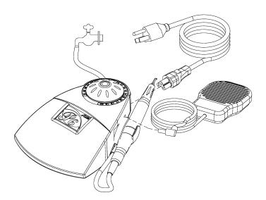
(Figure 2) System Installation Diagram
